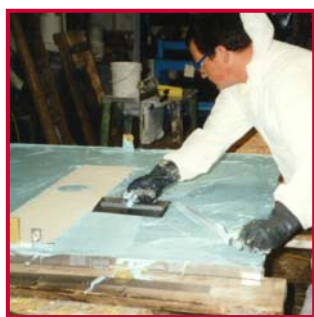
Preparing the Insulant and Intumescent test piece.
