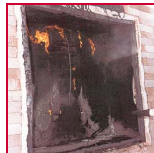
Jet Fire Test to the latest OTI 95 634 standard
